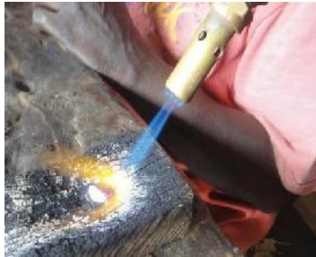
Figure 12: Melting pieces of silver scraps with a blow torch. Source: Emeriewen, 2014.
