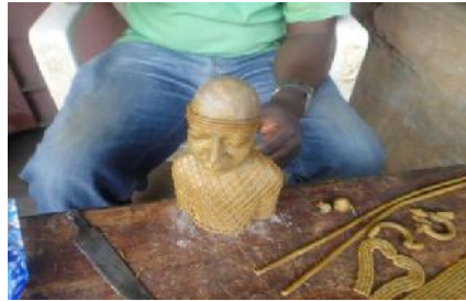
Figure 26: Covering up a core with beeswax Building-up (sculpting and ornamenting with strips and sheet of beeswax). Source: Emeriewen, 2014.
