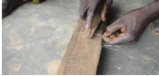
Figure 19: Twisting two strands of drawn wires together using a 2' X 4' wood with a flat piece of wood. Source: Emeriewen, 2014.
