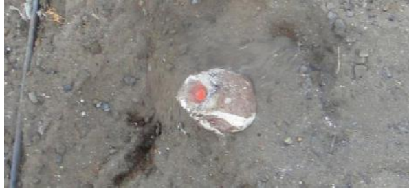
Figure 37: The iridescent mould buried halfway in the ground with the sprue positioned upward to receive the molten metal. Source: Emeriewen, 2014.
