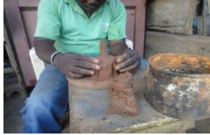
Figure 25: Making a core for a King's bust from well kneaded laterite soil. Source: Emeriewen, 2014.
