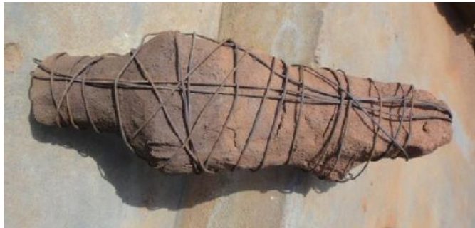
Figure 32: Carbon wire bound laterite soil casing (mould) of beeswax model. Source: Emeriewen, 2014.
