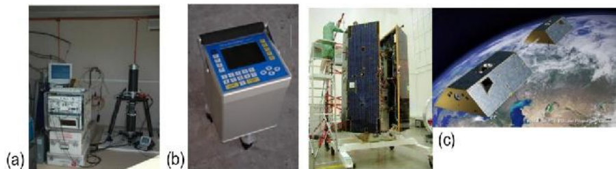
Figure 10 (a, b & c): Gravity Measuring Instruments and Tools [ (a) Micro-g LaCoste FG5 ( Absolute Gravimeter ); (b) Scintrex CG5 ( Relative Gravimeter ); (c) Gravity Satellites (GRACE 1&2)]
