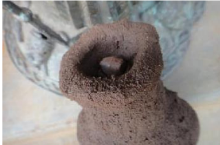
Figure 31: Addition of a sprue to the underside of the wax model. Source: Emeriewen, 2014.
