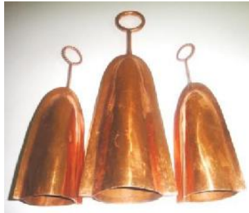
Figure 4: Copper gongs produced by sinking process. Source: Emeriewen, 2014
