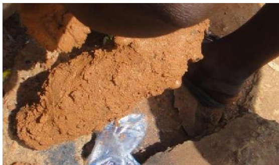
Figure 33: Covering the carbon wire bound laterite soil covering of beeswax model with slurry soil. Source: Emeriewen, 2014.
