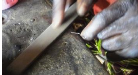
Figure 16: Filing an end of a silver wire for it to be drawn. Source: Emeriewen, 2014.
