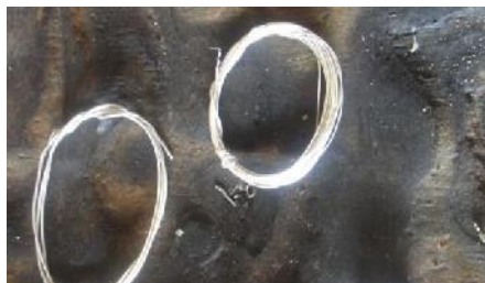
Figure 18: Drawn silver wires ready for use. Source: Emeriewen, 2014.
