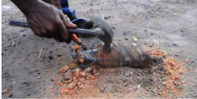
Figure 40: Destroying the laterite mould (casing) housing the metal cast. Source: Emeriewen, 2014.
