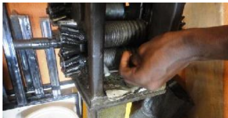
Figure 13: The melted silver in ingot form being reduced to thick wire form in a rolling mill. Source: Emeriewen, 2014.
