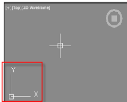
Figure 7: Coordinate points in a CAD template
