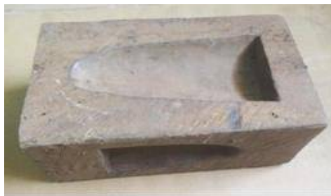
Figure 5: Sinking block used to produce the gongs in figure 4. Source: Emeriewen, 2014.
