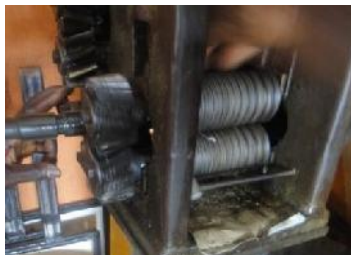
Figure 14: Further reduction of a silver wire in the tinnier grooves of a rolling mill. Source: Emeriewen, 2014.
