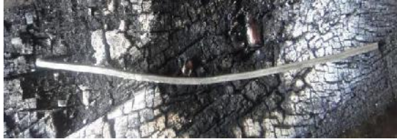
Figure 15: The reduced silver wire. Source: Emeriewen, 2014.
