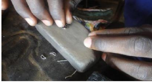
Figure 22: Using a Carborundum stone to file excess solder on the formed earring frame. Source: Emeriewen, 2014.
