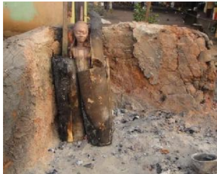
Figure 35: An open fireplace where moulds to be cast are de-waxed and warmed. Source: Emeriewen, 2014.
