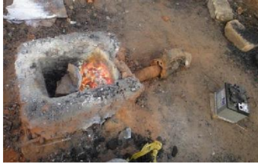
Figure 34: Melting copper alloy scraps in a furnace. Source: Emeriewen, 2014.
