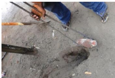
Figure 36: Placing a de-waxed mould (casing) in a dug hole. Source: Emeriewen, 2014.
