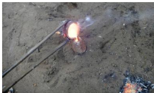
Figure 39: Pouring molten copper alloy into the mould to assume the shape of the expended beeswax. Source: Emeriewen, 2014.
