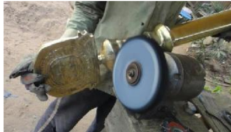
Figure 10: Polishing a mace with a charged polishing mop attached to an electric motor.
