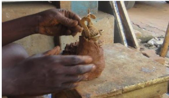
Figure 29: Covering the wax model with kneaded laterite soil. Source: Emeriewen, 2014.
